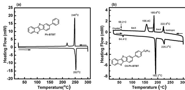
Fig. 3 DSC curves of Ph-BTBT and C6-Ph-BTBT.
