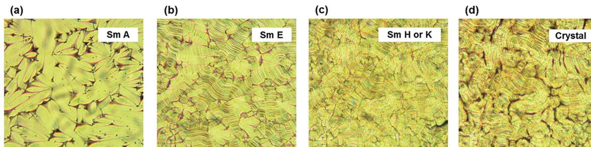
Fig. 2 Polarized optical microscopy images of C6-Ph-BTBT. (a) Sm A phase, (b) Sm E phase, (c) Sm K or H phase and (d) crystal phase.
