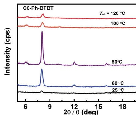
Fig. 6 XRD pattern of thin film based on C6-Ph-BTBT as deposited at various substrate temperatures.
