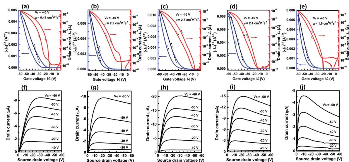
Fig. 4 Transfer and output curves of OTFTs of C6-Ph-BTBT films grown on an OTS-coated substrate at  $T_{\text{sub}} = 25$  °C (a, f), 60 °C (b, g), 80 °C (c, h), 100 °C (d, i), and 120 °C (e, j). (a), (b), (c), (d) and (e)  $I_{\text{D5}}-V_{\text{G}}$  characteristics curves; (f), (g), (h), (i) and (j)  $I_{\text{D5}}-V_{\text{D5}}$  characteristics curves.
