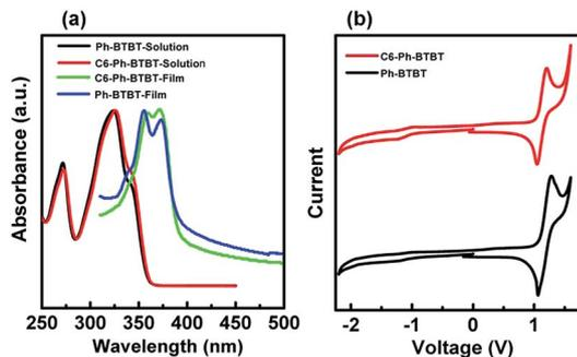
Fig. 1 (a) UV-vis spectra of Ph-BTBT and C6-Ph-BTBT; and (b) cyclic voltammogram of Ph-BTBT and C6-Ph-BTBT in dichloromethane.
