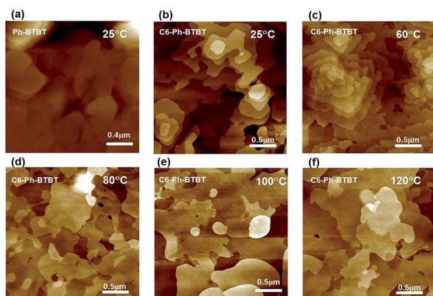
Fig. 5 AFM height images of thin-films. (a) Ph-BTBT as-grown film, and the films of C6-Ph-BTBT deposited at different substrate temperatures: (b) as-grown, (c) 60 °C, (d) 80 °C, (e) 100 °C, and (f) 120 °C.
