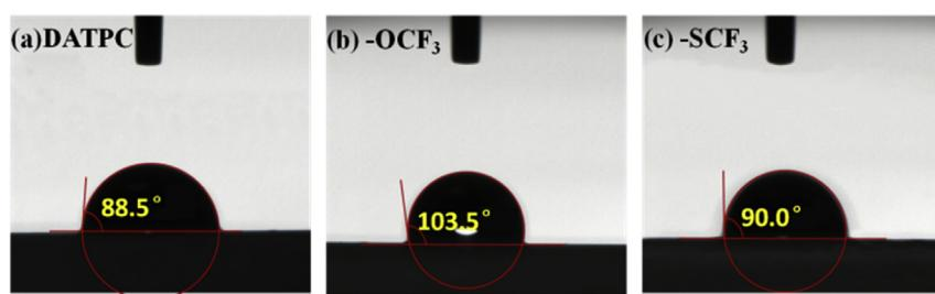
**Fig. 5.** Contact angles of (a) DATPC, (b) DATPC-OCF<sub>3</sub>, and (c) DATPC-SCF<sub>3</sub> measured by 2 μL water spread over vacuum-deposited 50 nm films on the glass.
