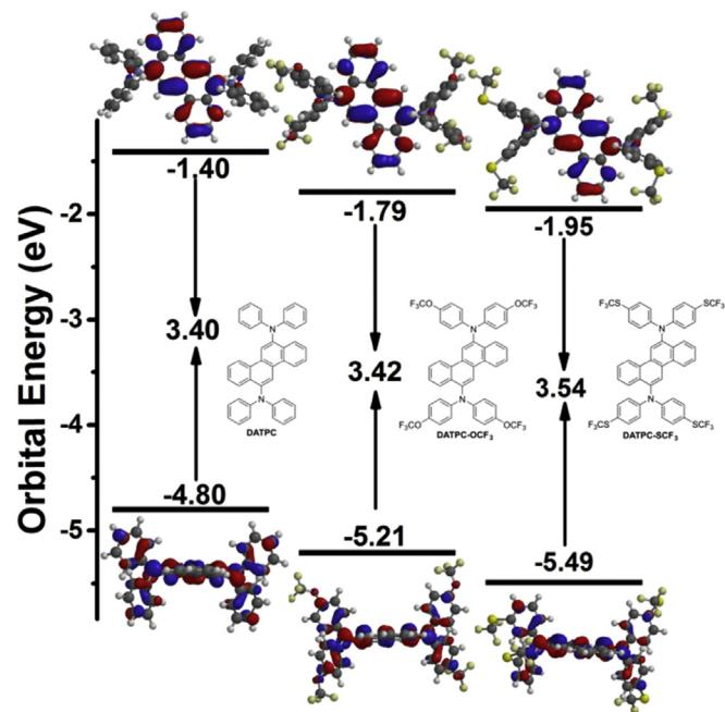
**Fig. 1.** Molecular structure; HOMO and LUMO electron density and orbital energy level at  $S_0$  state calculated by the DFT B3LYP/6-31G\* for DATPC, DATPC- $\text{OCF}_3$  and DATPC- $\text{SCF}_3$ .
