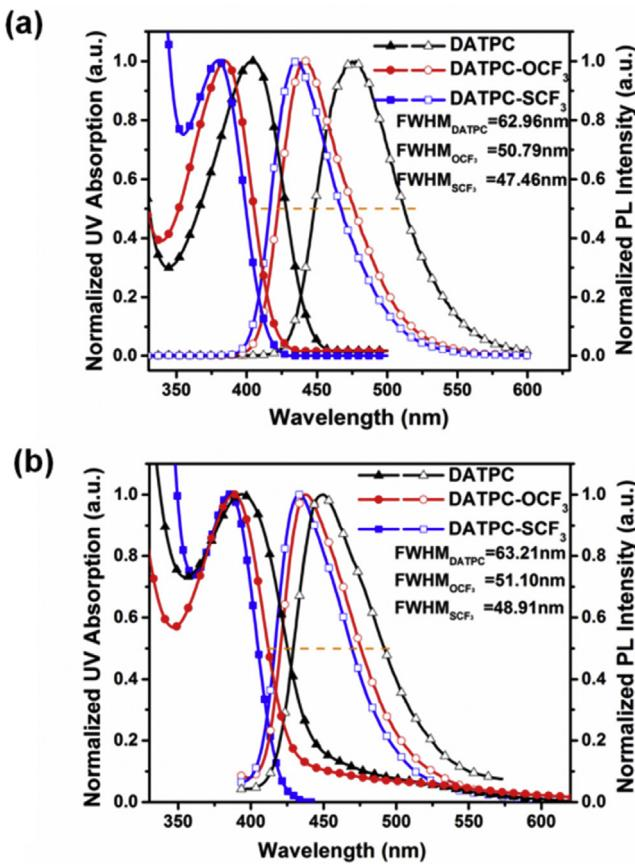
**Fig. 4.** The UV–vis absorption (solid dots) and fluorescence (hollow dots) spectra of DATPC, DATPC-OCF<sub>3</sub> and DATPC-SCF<sub>3</sub> (a) in anhydrous chloroform solution ( $1 \times 10^{-5}$  M); (b) in the vacuum-deposited films (50 nm) on glass substrates.
