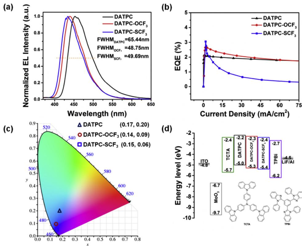
**Fig. 6.** (a) Normalized EL spectra of OLED devices made of DATPC, DATPC-OCF<sub>3</sub> and DATPC-SCF<sub>3</sub>; (b) External quantum efficiency (EQE) versus current density; (c) CIE coordinate; (d) Device structure of DATPC and its derivatives as blue emitters.
