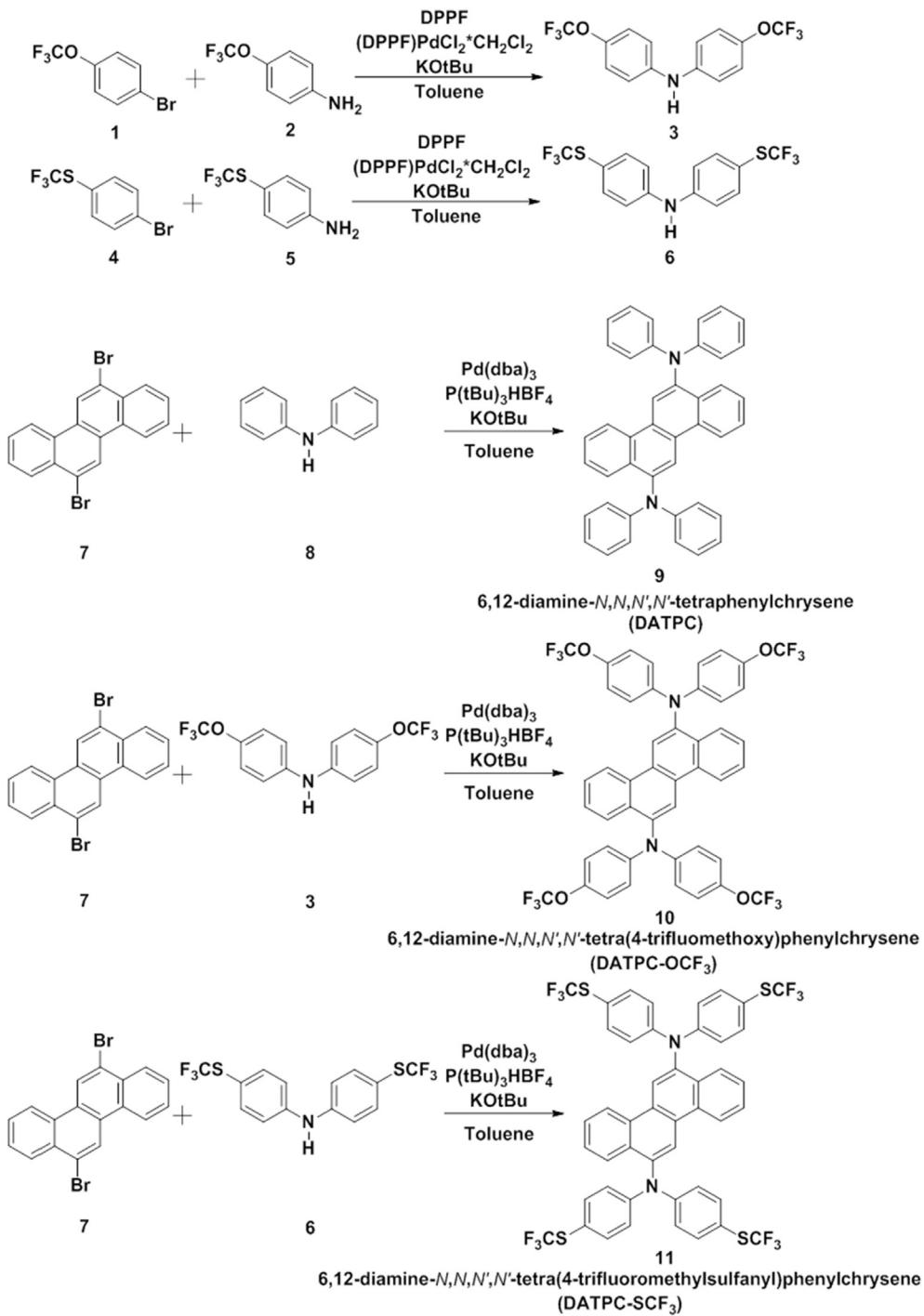
**Scheme 2.** Synthesis of 6,12-diphenylaminechrysene (DATPC) and its derivatives (DATPC-OCF<sub>3</sub> and DATPC-SCF<sub>3</sub>).
