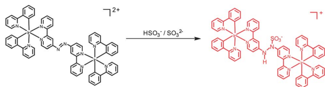
Scheme 2 Reaction of SP-2 with sulphite or bisulphite.
