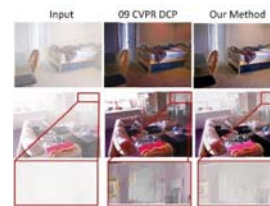
Fig. 1. The dehazing results with different methods. Our method can get clean results without color shift and blocking effect.
