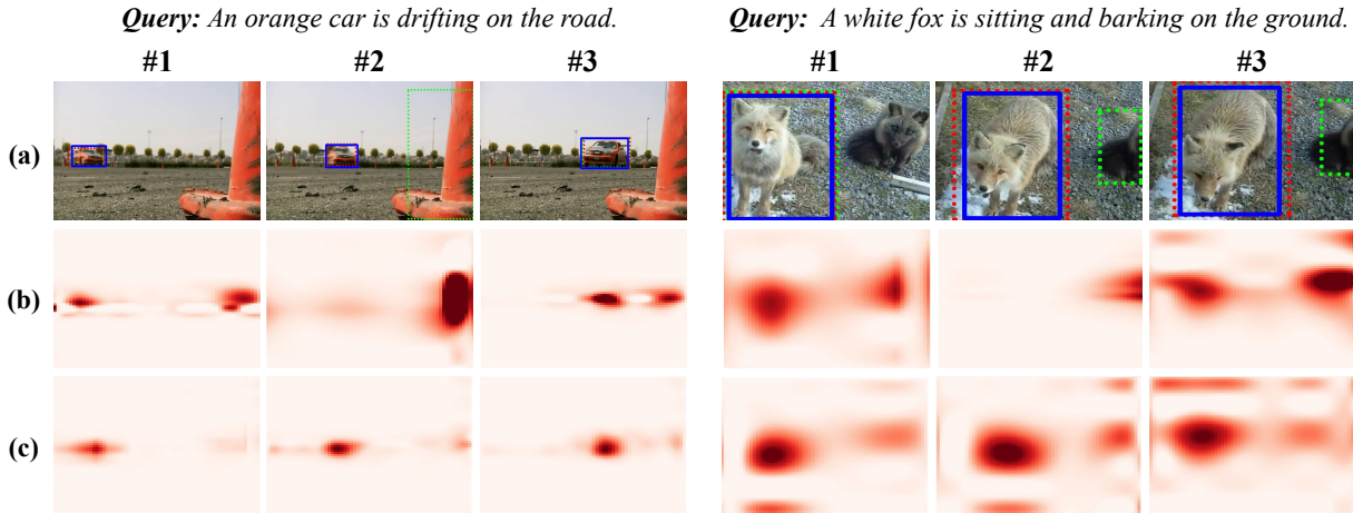
Figure 6: (a) Input image frames. Localization results of DCNet w/o and w/ the inter-frame contrastive loss \mathcal{L}_{inter} are marked in green and red, respectively. Ground-truth annotations are marked in blue. (b) Confidence score maps w/o \mathcal{L}_{inter} . (c) Confidence score maps w/ \mathcal{L}_{inter} . The score maps of DCNet w/ \mathcal{L}_{inter} are more stable across video frames than that of DCNet w/o \mathcal{L}_{inter} . Pay special attention to the #2 frame of the two examples.
